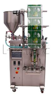
Automatic filling and sealing machine is suitable for all kinds of paste and liquid without gas, such as ketchup, sauce, oil and so on.
