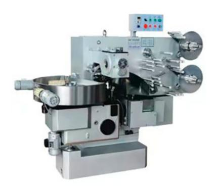
With sugar tray automatic material handling device, computer and photoelectric automatic detection and tracking, 100% packaging rate, no empty package, frequency conversion and speed regulation.
