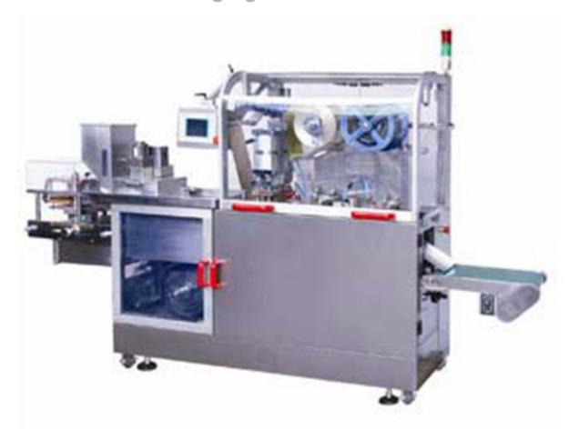
DPB140 Blister Packaging Machine is suitable for capsule, tablet, honey pill, candy, liquid (ointment), syringe as well as irregular shape Al-plastic or paper-plastic packing in pharmaceutical, healthcare, food, cosmetics, medical equipment industry etc. for for middle and small production.
