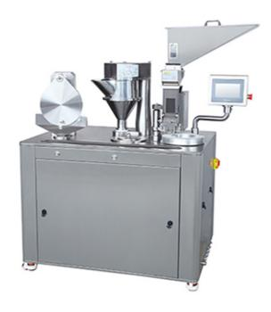
The semi-automatic capsule filling machine suitable for filling powder and pellet material in pharmacy and health food industry. it can meet laboratory require and low budget require.
