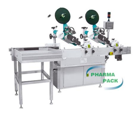
This machine is especially good for small round bottles working with high-speed labeling and high precision of labeling. Man-machine operation interface, any troubles will be displayed and inducted to remove. Simple operation, anyone can easily operate this machine. Intelligent label control and error warning functions. It is complied with GMP standard that provides easy maintenance and for a long durable life.
