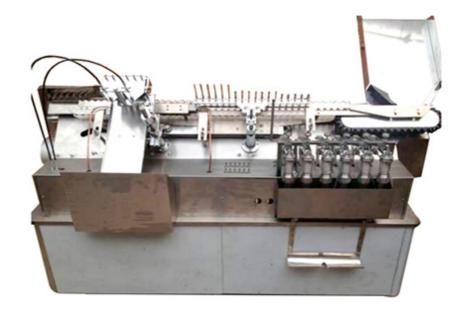
The machine is a new generation of the ampoule drawing, filling and sealing combined equipment for injections. It adopts the rectangular feeding instead of the traditional ampoule feeding methods. In such case, the feeding is steady with no easy broken ampoule. A modern clutch is mouthed under the ampoule feed hopper.
