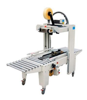
FXJ-5050Q tape-sealer is an automatic sealing of random-size carton boxes. The carton box must be introduced into the machine with the top flaps already closed: the upper taping head and the side driving belts automatically adjust to the box dimensions. The top and the bottom flaps are simultaneously sealed. Ideal solution for carton boxes with a maximum 50-cm width and height.
