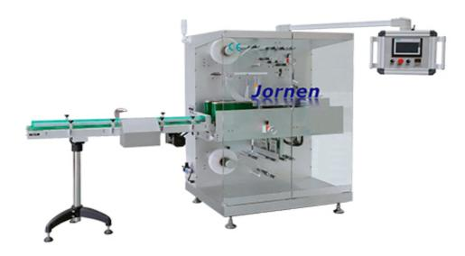
The Stretch-Banding Machine is an End-of-Line Packaging Machine. It can group together or stack cartons (or similar shaped objects) to form larger units. These are then tightly wrapped in plastic film. Compared with shrink-wrapper and overwrapper, this machine is energy-saving as it does not require heating up. It saves 50% of film materials because it partially covers the packaging. It can be connected to a packaging line with Blister Machines, Cartoners, and Case Packers.
