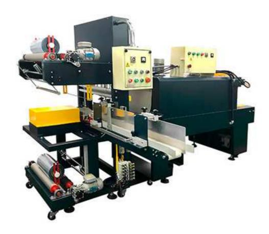
Sleeve-type Sealer with Tray Model, SSA1400 & SSA-1600 has PLC control system can detect film running and alarm of trouble to indicate problem helping technician fix machine easy.
