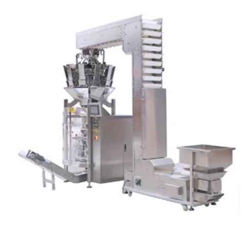
Automatic bayonet weighing hopper, storage hopper, main vibration and wire vibration without screw fixation. Simple disassembly and convenient cleaning.
