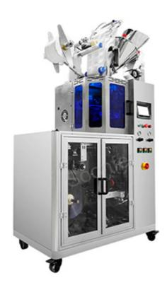
Drip bag coffee packing machine suitable for inner and outer bag packaging for suitable to package coffee powder, tea powder and tea leaves.
