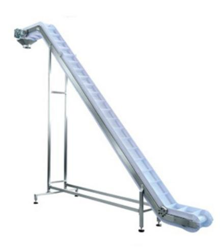
L-shaped Conveyor is made of stainless steel sanitary construction and food grade polypropylene (PP) belt, with good appearance, not easily deformed, bear high and low temperature. The conveyor allows for controlled feeds at one or more locations and can easily interface with various types of feeding devices.
