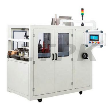
Horizontal storage is adopted for storaging carton blanks, for which carton blanks can be added at any time without stopping the machine
