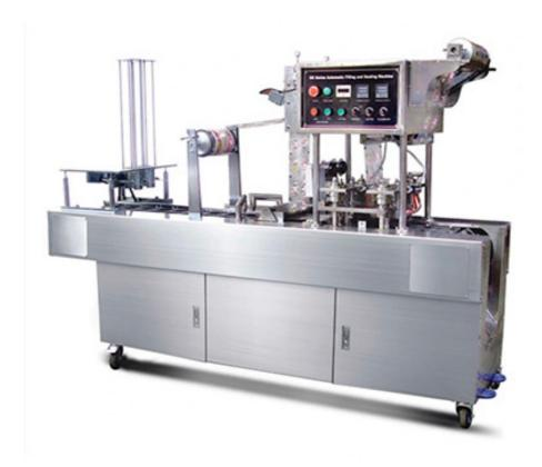
BG32A (2 cups)/BG60A (4 cups) automatic cup filling and sealing machine is widely used in filling and sealing various kinds of plastic cups for liquid.
