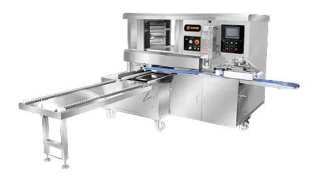
The STA-360 Automatic Stamping and Aligning Machine is the solution for automatically shaping, stamping, and aligning food on trays, which can make various snacks such as mooncake, pineapple cake, and maamoul. The stamping mold can be customized as needed.
