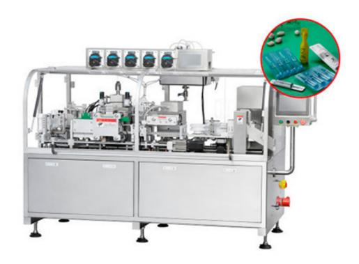
The DC-860 double-sided blister machine is mainly a filling machine for metering and packaging liquid and semi-viscous products. This product is designed to meet the needs of liquid and semi-viscous product packaging using plastic roll film. The production line is simple, safe, and can reduce product production costs. Modular design, simple structure, short design cycle, and fast product updates. Reasonable structure, reliable quality, stable operation, and long service life.
