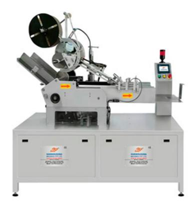
The Automatic Carton/Pouch Sticker Labeling with Stacker system consists of a main structure, stacker for product holding, product transmission belt with guide adjustment, label dispensing unit, label pasting by nylon brush & sponge roller, motors, sensors, electrical panel, PLC & HMI (Keypad), AC drives & mains ON/OFF.
