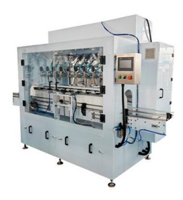
This machine is specially used for filling corrosive liquids or chemicals, and is suitable for oil, paint, ink, and curing agent, adhesive, organic solvent, cleaning agent, diluent, resin, polyurethane, pesticide, medicine, lubricant and various flow able liquids.
