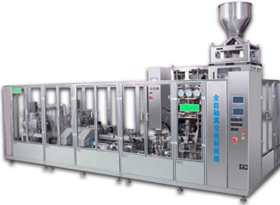
This machine including one set automatic vertical bag making packing and sealing machine one set linear weigher, One set vacuum packing machine, one set output conveyor. This machine are widely use for packing food pharmacy chemical and other granules, Like coffee beans, yeast powder and so on. The whole machine adopting inside pumping to vacuum product. The vacuum degree is very high and packing speed is very high, the finished product is very nice and have a long shelf life.
