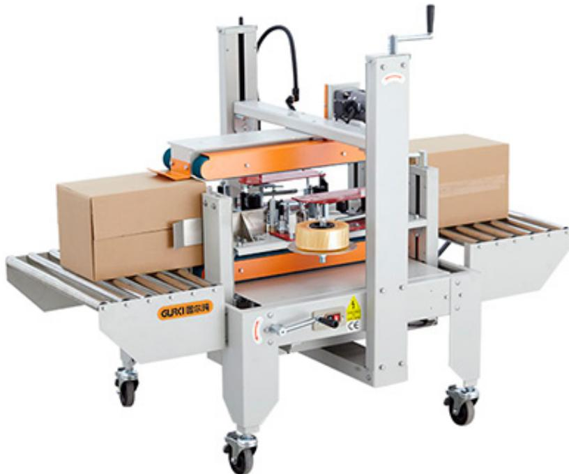
Two sides sealing machine GPS-50 is characterized in that the carton is placed sideways to seal the upper and lower sides of the carton, and is suitable for cartons with side openings, such as beverages, floor tiles, and the like. The sealing result is flat, standardized and beautiful. This machine, which is economical and easy to adjust is sealed with tape.
