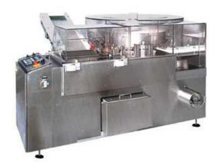
The SD-CT-16 ultrasonic bottle-washing machine can be used as inside bottle washing as well as outside bottle washing. Bottles such as oral taken bottles, mould bottles, medicine bottles can use the machine. It is equipped with electricity controlling system. The equipment can work independently or be used to work with a whole line that connected to other machines to form a set of production line.
