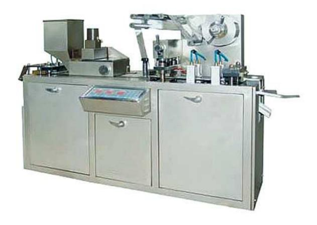
Automatic machines for the packaging of tablets in blister pack used for the packaging of different sizes of containers with honey, coated tablets, capsules and vitamin. Due to its size, it can also be used in plastic-packaged in aluminum blisters and aluminum packaging for chocolates, small computer parts, etc. Currently, equipment is widely used in the pharmaceutical, hospital and college laboratories and worksites for testing of small engines.
