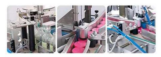
The A107 uses a pneumatic fork to hold the bottle for rotation and is particularly suitable for large diameter and heavier bottles. Designed for wrap-around labeling on relatively large and heavy bottles with orientation features; also capable of putting two labels on one bottle. Using a pneumatic arm for bottle holding, and 3 point rotation method, extra label alignment and registration precision are ensured.
