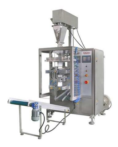
This fully automatic packaging machine that is designed to prepare 4 side sealed sachet-type packages, and to place untouched non free flowing powdered products.
