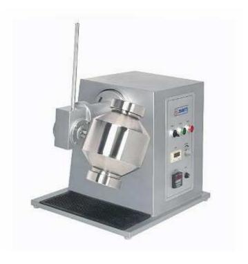
Double Cone Mixer operates on free flow principle. This unit is used for rapid mixing of all types of free flowing powders and granules. The uniform, multidimensional arrangement of the mixer walls ensures good mixing. The vessel is manufactured from stainless steel and secured with threaded knobs. This unit can be attached to the Universal Gearing.
