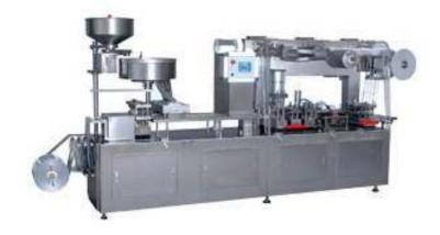
The DPB-140 blister packaging machine is widely used in small pharmacy factory, dosage room of hospital, research institute of hardware factory, food products factory, health products factory and pharmaceutical factory for troche, candy, icing, milk tablet, packing capsule, little hardware etc with Al-Foil.
