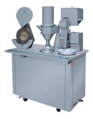
The machine is a new type of medicine packing machine with novel structure and attractive appearance. Under both electrical and pneumatic control and equipped with an automatic electronic counter and computer-controlled speed-adjusting device, the machine can accomplish the positioning, separation and locking etc. of capsules. In place of manual capsule-filling, it can reduce labor intensity and up to sanitary standards for pharmaceutics.
