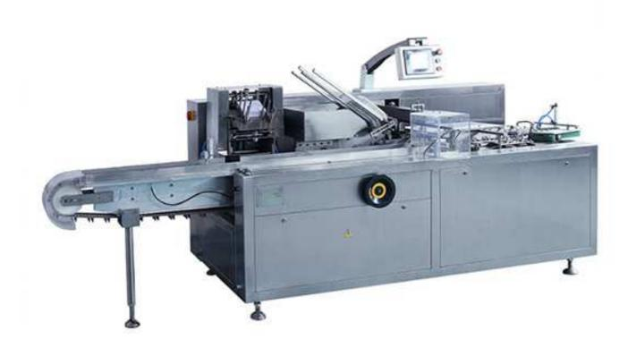
This machine is suitable for automatic cartoning of tube, ointment and soft package. It consists of direction folding (1-4 folds) and feeding equipment, carton forming and feeding, batch number printing, sealing of case tongues at both ends etc. The whole cartoning process is finished automatically. It can be added with hot-glue device for the carton sealing.
