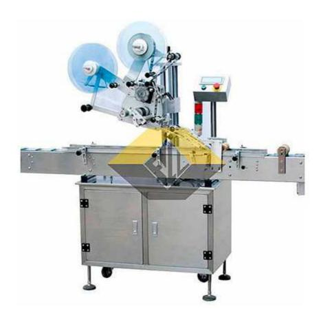
Planar Self-Adhesive labeling machine is applicable for the surface labeling for various paper boxes, cartons, batteries, cosmetics and etc, such as anti-counterfeiting labels, bar codes so on.
