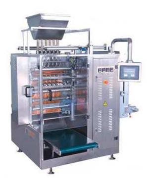
As shown in the picture, the granule packing machine is used for packing loose, non sticky granule materials in the medicine, food, daily chemical and other industries. It can be applied to measuring and automatic packing into sachets such materials as Chinese medicine infusion, oatmeal, coffee, etc., crystalline materials like monosodium glutamate, white sugar, salt, etc. and small shot materials like Chinese patent drugs, dryers and so on.
