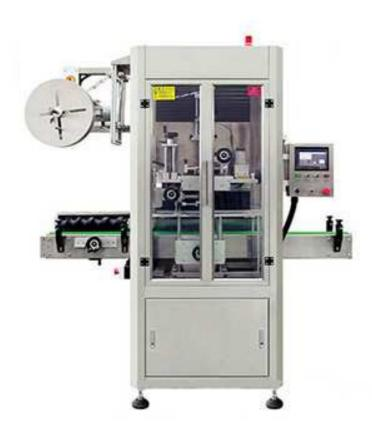
The machine adopts advanced international technology to insert and sealing the shrink label on round or square bottles.
