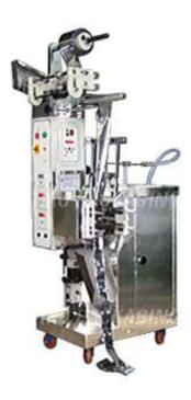
The MK-102 is an automatic small vertical form fill seal packaging (VFFS) machine designed to package liquid and semi-viscous products. This machine uses volumetric piston dosing system and is integrated with continuous type sealing system to produce 3 side sealed and 4 side sealed pouches / bags.
