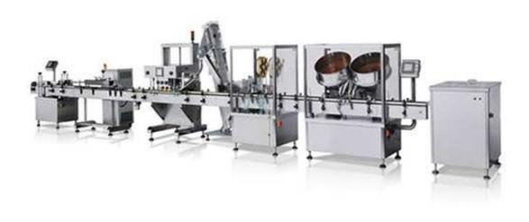
This line includes bottle unscrambler, capsule counting machine, desiccant inserting machine, screw-capping machine, induction sealing machine and labeling machine, which all line is in accordance with the requirements of GMP.
