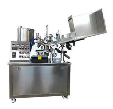
This machine is mainly used for Plastic & Laminated tube filling and sealing.
