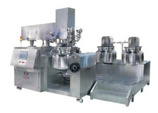
The Hydraulic lifting vacuum emulsifier is the ideal equipment for the Cosmetic, Skin care, Daily chemical and Food industries. The high shearing homogenizer, make the raw material distribute equally. The material of our machine adopt high quality Stainless steel SUS304 and 316L, safety and durable.
