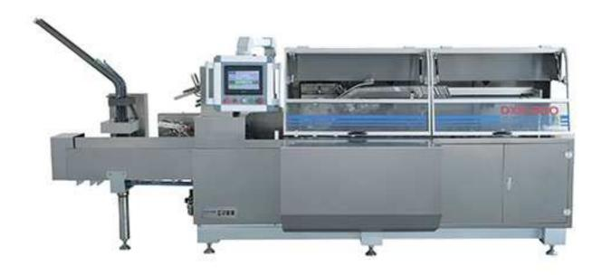
DXH-200 High Speed Automatic Boxing Machine belongs to the continuity, high speed, incorporated pneumatic-photo-electro-mechanic high technology products. The machine is suitable for automatic feeding and packing products, such as ALU-PVC blister, bottle, cosmetics, commodity, hardware, card, and some other similar products into the carton, which can automatic finish the leaflet folding, carton opening, feeding, printing lot number, sealing, etc.
