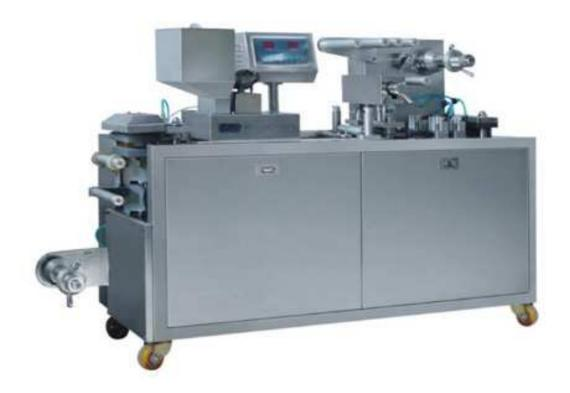
It is the newest high precision capsules and pills/tablets packing machine in current pharmacy industry. It is widely used for capsule, tablet, honey pills in pharmaceutical industry, for milk tablet, candy, chocolate in food industry, for injector, syringes, pins, small component ect. In electron or hardware industry as all kind of shapes of ALU-ALU, ALU-plastic, paper-plastic combined packing.
