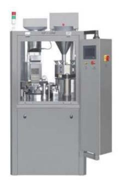
SED-1200J adopt PLC control system, human-machine interface, when running malfunction or lack of stuff, automatic alarm, malfunction display, automatic dismiss alarm. And with functions of password setup, touching screen display, automatic parameter setup, data printing, reset, etc.
