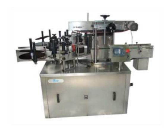
Pack Well is Automatic Vertical Sticker Labeling Machine is one of the most users friendly. The machine is used for two sides labeling on flat surface of different size of flat container. It is capable to labeling up to 150 containers per minutes depending on products and label size. The automatic model is equipped with belt spacing device resulting in a simple to "No change parts required".
