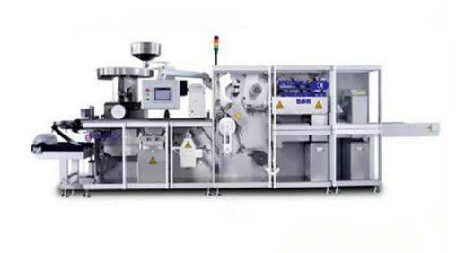
KWDPH320H II -S full Servo Roller Type High Speed Blister packing Machine, the fastest can complete 720 Blister/min. Through the digital HMI multi-task production mode, the super high speed roller type AL/AL blister packing can be achieved.
