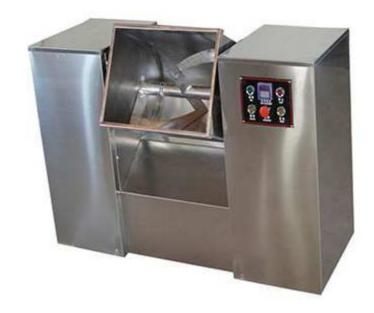
Ribbon Mixer comprises of a U-shaped horizontal trough and a specially designed Double Helical Ribbon Agitator rotating within. Ribbon Mixers are based on a proven agitator construction that provides a triple mixing action ensuring fast, efficient blending. The dimensions and configuration of the ribbons are carefully balanced to provide a movement of material within the container that avoids dead spots and gives rapid product discharge.
