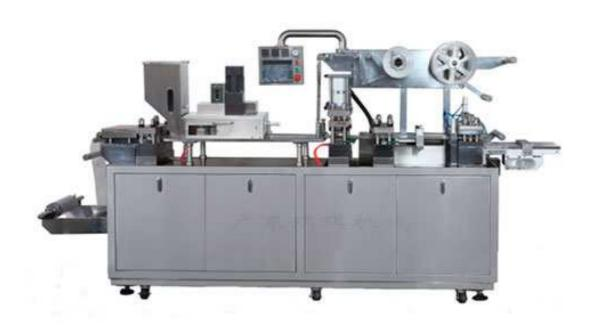
DPP-320E Model Flat Plate Auto Blister Packaging Machine is suitable for aluminum-aluminum, aluminum-plastic, paper-plastic.
