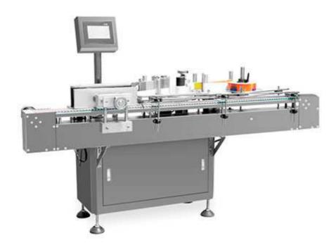
Abel pre-feeding system makes the label feed stable, stickup smoothly and label position precise. Equipped with human-computer interface and PIC control system, Ensure more stable operation and easier handling. Label-feeding adopt tension design to ensure that the coding quality, and can accurately control the length and uniformity of the label. The label-rolling and label pressing adopt different structure by different bottles shape to ensure the quality of the labeling.
