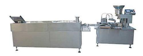
As an incorporated body of washing, drying and filling, this oral liquid production line is specially designed for washing, drying, filling, capping and sealing 10ml or 20ml linear glass bottles with easy open lids.
