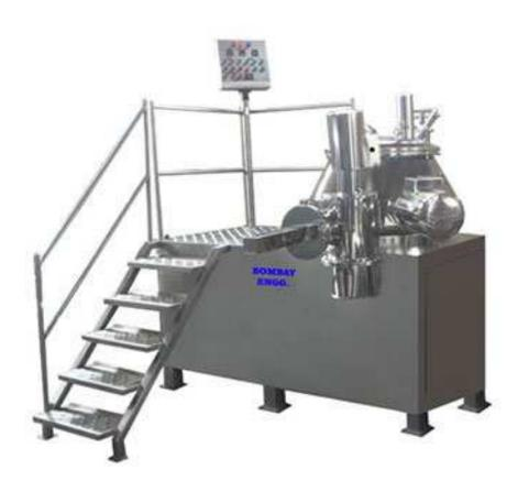
Rapid mixer granulator is a multi-purpose processor equally suitable for high speed dispersion of dry powders, aqueous or solvent granulation, and effervescent products and melt pelletization.
