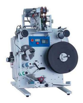
Powerful, single-label, double-label labeling function can be switched at will, the distance between the front and the double standard can be flexibly adjusted, and the circumferential positioning function can be selected to set the position label on the circumferential surface;
