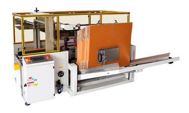
The machine is suitable for paper carton erecting automatically. It has function of cover-folding, sealing bottom with tape. It is economical and it is with high high-efficiency. It is ideal automatic carton forming and bottom sealing equipment.
