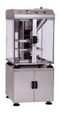
DP-12 model single tablet press machine is to absorb advanced technology successfully developed. It is pharmaceutical, laboratory and other industries first choice and able to press the powder and granular material into tablets continuously and automatically.
