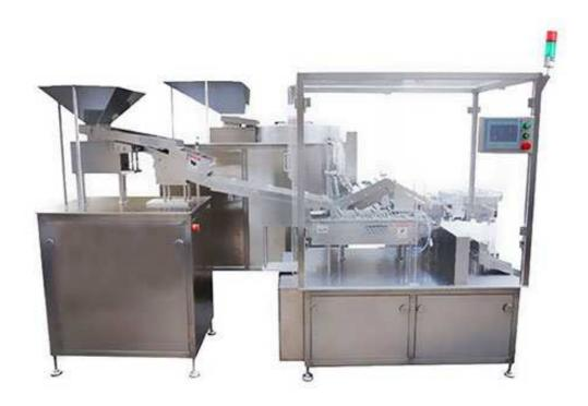
The BSP-60A Straight-Tube effervescent tablet Filling Machine is applicable to the packing bigger and thinner tablets which are orderly fed into bobbin bottles in single row in an overlapping way. The device utterly adopts a PLC for centralized control, it is verified in fiber and photoelectric detections and other kind of detections to have steady performance and reliably automatic operation. It can automatically give alarms and shut down in case of no tablets, bottles or covers.
