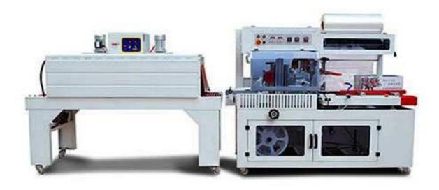
PZS-950L automatic heat shrink packaging machine is a fully automatic unmanned operation "L" automatic shrink packaging machine, widely used in food, pharmaceutical, daily chemical, hardware, electrical and other industries, especially mass production. Packing flow operation, high work efficiency, automatic film feeding and punching device and manual adjustment of the film guiding system and manual adjustment of the feeding platform for different widths and heights.
